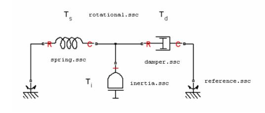
The domain is declared in a file named rotational.ssc (see "Declare a Mechanical Rotational Domain" on page 2-20). The following file, named spring.ssc, declares a component called spring. The component contains:
